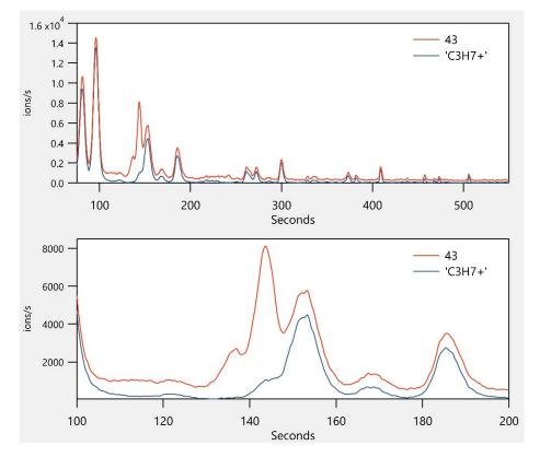
Figure 2. A full chromatogram from the GC-EI-ToF instrument (top) showing two ions with a mass-tocharge ratio of m/z=43. A zoomed-in view (bottom) is also shown.
